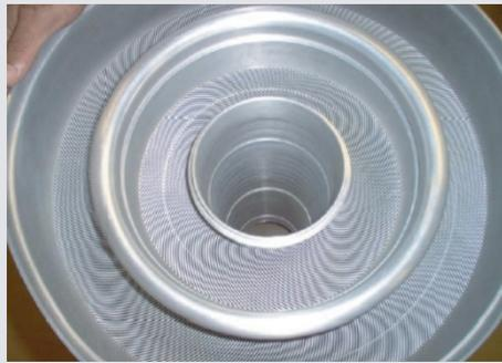
The unique fuel assembly design for the High Flux Isotope Reactor (HFIR)
